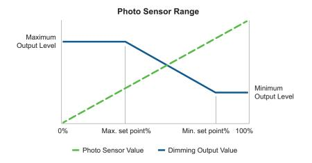
The rate that dimming output changes is defined by the parameter *open loop dimming rate* which defines the time for dimming to go from 0% to 100% or vice versa (default 65 seconds).
