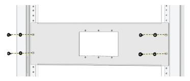
2. Align the mounting collar to the rack-mount panel with the arrow directed up (as shown below), and secure it in place using three mounting screws (provided with the controller).
