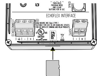
3. Cycle power to the unit. The INPUT STATUS, LEARN/TEACH, and PROGRAM MODE LEDs flash to indicate the update process has begun. After several seconds, the OUTPUT STATUS LEDs illuminate to indicate the progress of the update.
