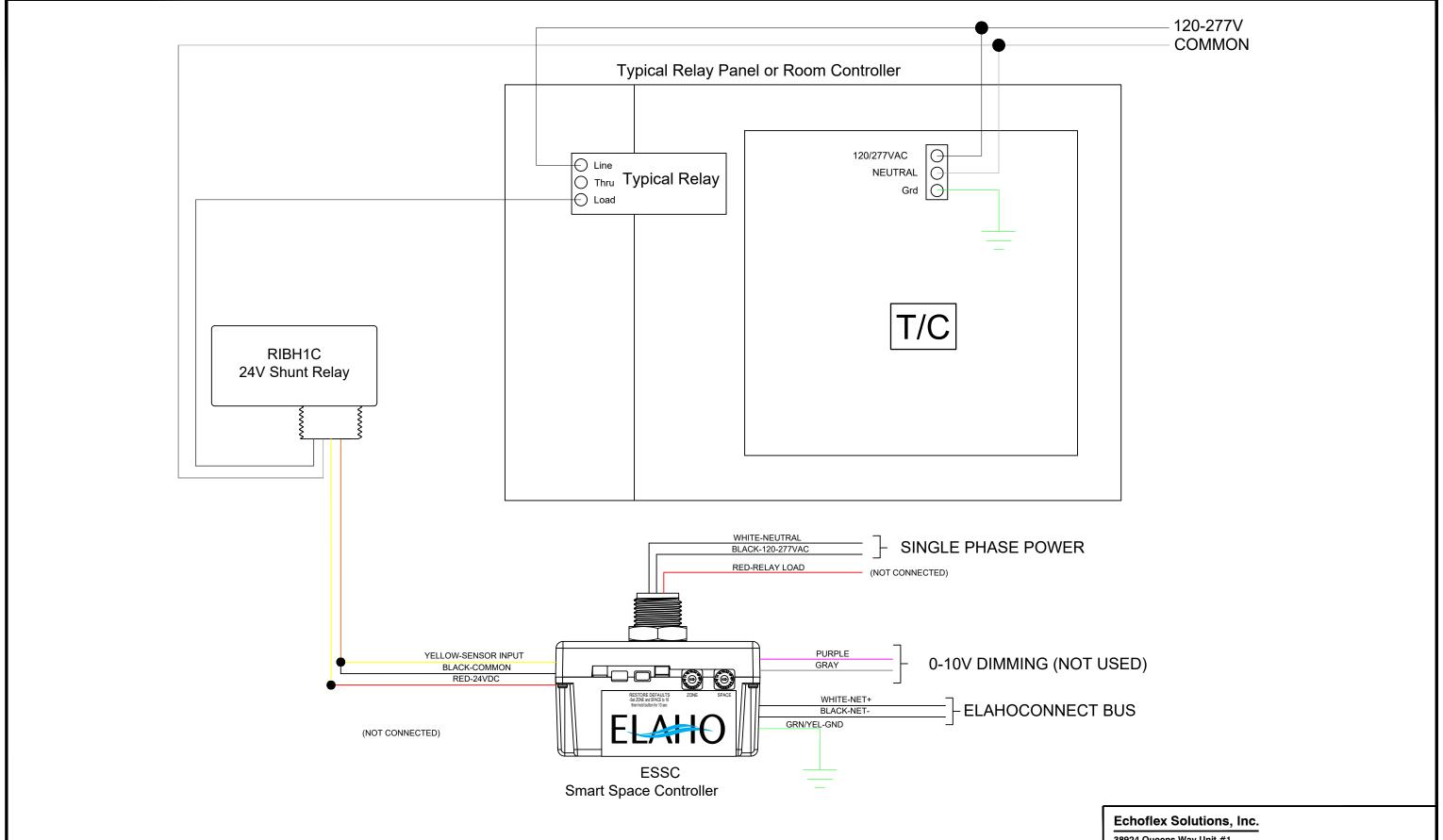
Typical Wiring Diagram - ELAHO SMART SPACE CONTROLLER (ESSC)
