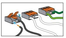
Terminate EchoConnect wiring using provided WAGO connectors.
