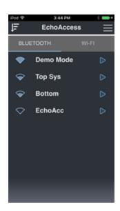
Selecting an Access BT Interface from the list connects to the Elaho control system and displays the **Preset Control** page where you will be able to control presets and zones for each **allowed space**. See **Preset Control on page 15** and **Allowed Spaces on page 32**. The number of spaces configured for the Elaho control system is indicated by dots on the bottom of the **Preset Control** page. Swipe the page to the left or right to access additional spaces.
