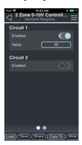
Swipe to the left or right to access the Demand Response page and enable or disable demand response for each circuit. Enter a **Value** between 0 and 99 to set the highest output level when Demand Response is Enabled.
