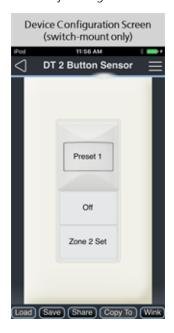
Tap on a button to configure its actions. To configure the occupancy sensor, see **Configuring the Occupancy Sensor on page 48**. The selected control's Configuration page displays. Additional menu options will display based on the *Action* selected (e.g., if the Push *Action* is set to Preset Activate, Preset Number and Timing (in seconds) displays for specification).
