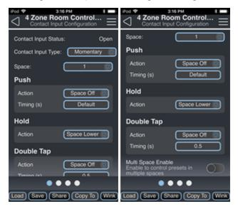
The *Multi Space Enable* switch will display if the **Push** *Action* is set to Preset Activate, Preset Toggle, or Space Off, allowing you to choose multiple spaces to which that action will be applied.
