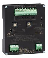
Elaho Demand Response Interfaces are DIN rail mounted devices that accept four maintained closures to trigger demand response within an Elaho control system.
