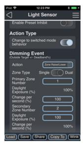
**Daylight Exposure (%)** is set to 100% for the Primary Zone Number and cannot be changed. The Primary Zone Number has the highest possible capacity for ambient daylight exposure and this is the location where the Light Sensor will be sampling light. The Secondary Zone Number Daylight Exposure (%) setting is user configurable.
