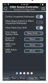
Use the available drop down menus and keypad to specify the desired configuration information. Additional configuration options will display depending on the selected action. For example, if the **Power On Behavior** is set to Preset, Preset Number will display for additional specification.
