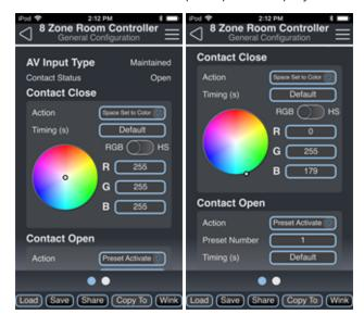
Use the drop down menus and keypad to set the **Contact Close** and **Contact Open** *Actions* and any additional options that display according to the actions selected.
