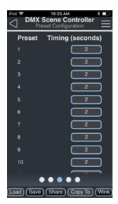
The Preset Configuration page allows for the configuration of each local preset's fadetime. This is the time that the preset will take when activated or deactivated.
