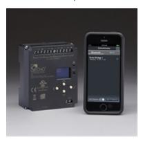
The Expansion Bridge also allows connection of up to four individual Elaho segments (control systems) so more control stations and Responsive Controls can be used within an Elaho control system. Each segment supports 16 power controllers and up to 16 Elaho devices (stations or responsive controls). Expansion Bridge integration enables Elaho segments to share spaces, presets, and zones.
