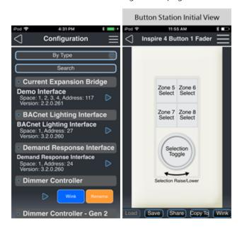
Winking a device causes the device to respond by blinking its local LEDs, and for certain devices its connected loads, 8 times over 16 seconds. Wink will auto-clear after 16 seconds and return the device to its normal operation. Using the device's local UI buttons or asserting control during the wink cycle disables wink, restores the previous look, then fades to the new control values.
