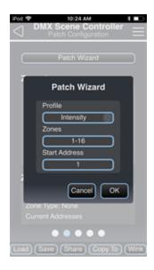
Tap the [Patch Wizard] button on the Patch Configuration page to patch multiple zones using the same Profile settings.
