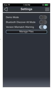
• [Manage Files]: Tapping this button opens a list of saved configuration files. Buttons at the bottom of the list allow you to share or delete files.
