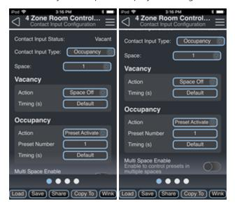
Use the drop down menus and keypad to set the **Vacancy** and **Occupancy** *Actions* and any additional options that display according to the actions selected. The *Multi Space Enable* switch will display if the **Vacancy** *Action* is set to Preset Activate or Space Off and **Occupancy** *Action* is set to Preset Activate, allowing you to choose multiple spaces to which these actions will be applied.
