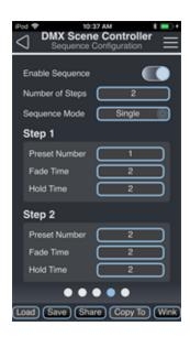
The Sequence Configuration page allows for the configuration of one sequence that plays presets in a predetermined order.
