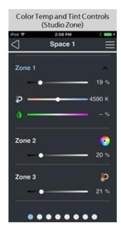
• Use the slider or tap on the number to the right of the slider and use the keyboard to enter a value for tint. The range of tint is 0-100.
