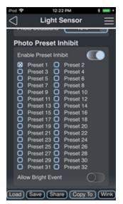
Allow Bright Event (switched mode) and Allow Lower Event (dimmed mode) - when this switch is enabled, lower or bright actions will not be affected by Daylight Exempt Presets, but raise and dark actions will be inhibited. When this switch is disabled, all raise, lower, bright, and dark actions will be inhibited by the Daylight Exempt Presets.
