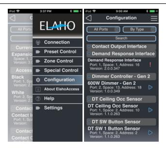
Configurable devices display a blue arrow on the right side of the device name. Devices in the list with a duplicate address will indicate with a red exclamation point on the right side of the device name.
