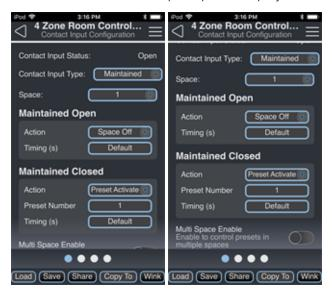
Use the drop down menus and keypad to set the **Contact Closed** and **Contact Opened**Actions and any additional options that display according to the actions selected. The Multi
